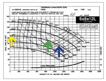
A correct pump curve is required to establish a baseline for pump performance.
