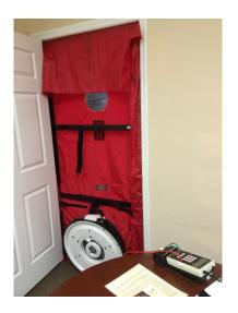
Building Enclosure Testing is a value-added diagnostic procedure that identifies how much a building leaks air. The higher the rate of leakage correlates directly to higher energy costs.
