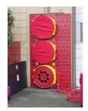
against the outdoor air pressure. After the building's internal air pressure is reduced, areas of leakage draw air into the building due to the negative pressure difference between indoor and outdoor air.
